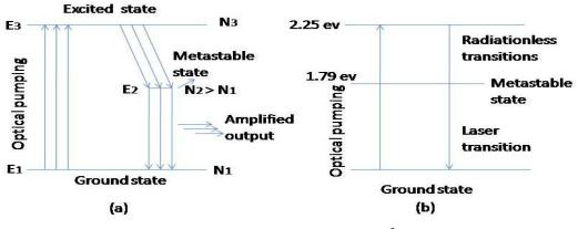
**Fig. 1.9** Energy level diagram of  $Cr^{3+}$  ions in ruby
