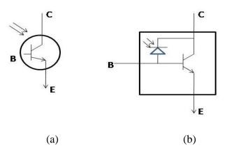
Fig.4.22 (a) Circuit symbol (b) Equivalent circuit of Phototransistor
