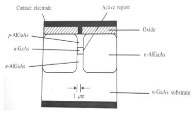
Fig.3.28 GaAs / AlGaAs buried heterostructure device
