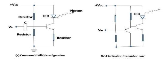
Fig.3.10 Transconductance drive circuits for analog transmission
