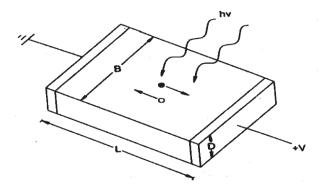
Fig.4.9 Sketch of photoconductive device
