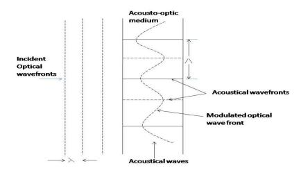
Fig. 4.6 Schematic illustration of acousto – optic modulation. The acoustic waves change the refractive index of the medium in a periodic way so that the plane optical wavefronts take on the 'wavy' appearance shown (very much exaggerated) as they propagate through the medium.
