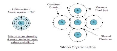
**Fig.2.1 A Silicon Atom Structure**
