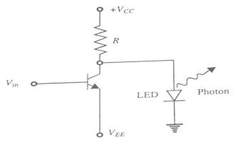
Fig. 3.14 Low impedance drive circuit consisting of a simple shunt configuration.
