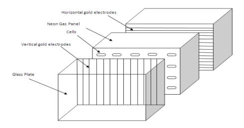
Fig.5.4 Architecture of Plasma Panel Display
