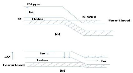
Fig.1.15 Heavily doped p-n junction (a) in equilibrium and (b) with forward bias.
