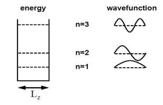
Fig. 2.13: Infinite quantum well and associated wave functions.
