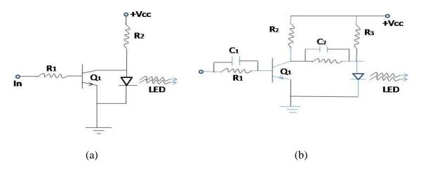
Fig.5.3 LED drive circuits (a) Simple circuit (b) Improved version of (a)
