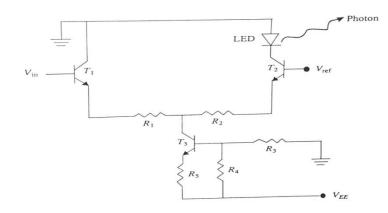
Fig.3.11 A differential amplifier drive circuit
