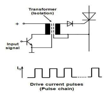
Figure 5.2. Principle of a thyristor driver circuit
