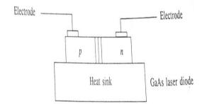
Fig. 3.19 A simple *p*-*n* junction diode
