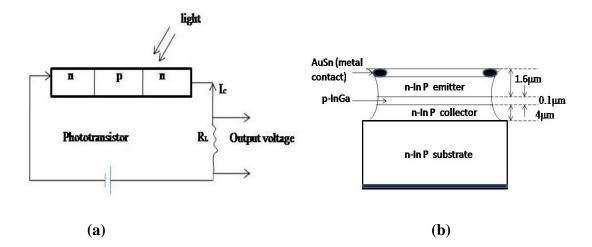
Fig.4.21 (a) Structure of homojunction phototransistor (b) heterojunction phototransistor
