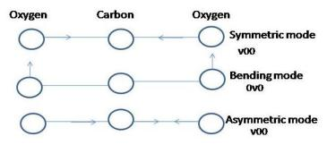
Fig. 1.13 Vibrational modes of the CO<sub>2</sub> molecule
