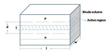
Fig.1.16 Diagram showing the active region and mode volume of a semiconductor laser
