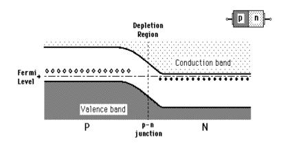
**Fig.2.6 Energy Diagrams of PN Junction**
