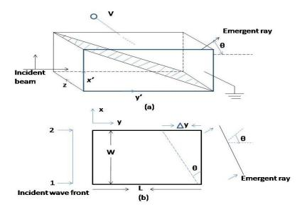
Fig 4.4 Schematic diagram of a beam deflector : (a) the double –prism KDP beam deflector and (b) the principle of defelction beam in a medium where the refractive index varies linearly in a direction normal to the direction of propagation.
