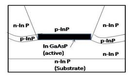
Fig.3.23 Cross-section of a buried heterostructure semiconductor laser
