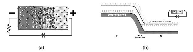
Fig.2.8 Biasing the PN Junction. (a) Reverse bias (b) Energy band diagram
