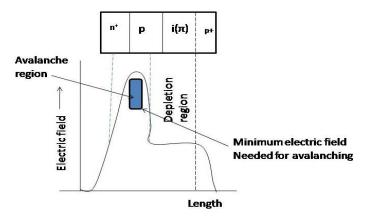
Fig.4.17 Avalanche photodiode in the avalanching mode.
