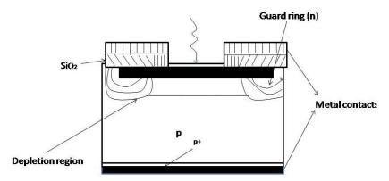
Fig.4.18 Silicon avalanche photodetector with guard -ring structure.
