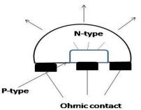
Fig.3.4 The structure of a hemispheric LED
