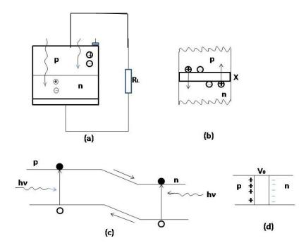
Fig.4.26 (a) p-n junction solar cell with load resistance,  $R_L$  (b) Diffusion of electrons and holes (c) Energy band diagram corresponding to (b) and (d) Formation of the open circuit voltage  $V_0$
