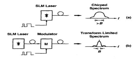
Fig. 3.1 Optical transmitters: (a) direct modulation vs. (b) external modulation
