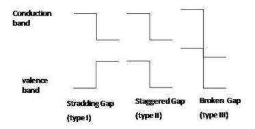
Fig. 2.9 Three types of semiconductor heterojunctions organized by band alignment
