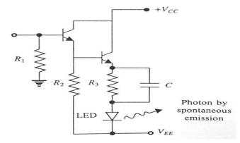
Fig.3.13 Low impedance drive circuit consisting of an emitter follower with compensating matching network
