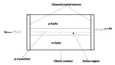
Fig.3.24 Schematic diagram of a GaAs heterojunction injection laser with a Fabry-Perot cavity
