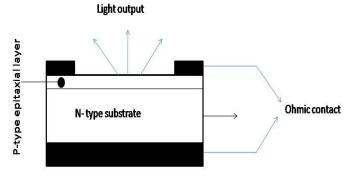
Fig3.3 Planar light emitting diode
