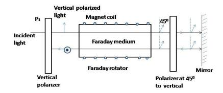
Fig. 4.5: Optical isolator based on the Faraday effect. The reflected ray is shown displaced for clarity.
