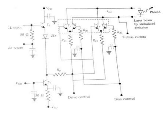
Fig.3.18 An ECL compatible high speed laser drive circuit
