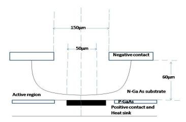
Fig.3.6 Axial cross-section through a Burrus-type surface -emitting LED
