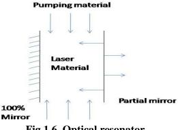
Fig.1.6 Optical resonator
