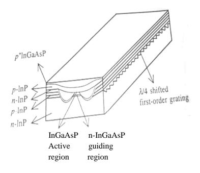
Fig.3.31 Quarter wavelength shifted double channel planar BH-DFB laser
