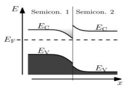
Fig. 2.10 Band diagram for straddling gap , n-n semiconductor heterojunction at equilibrium
