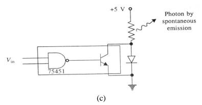
Fig.3.15 (a) Interfacing of the LED drive circuit with logic input levels (b) A simple TTL compatible LED drive circuit employing 74S140 line driver (c) A TTL shunt drive circuit using integrated circuit
