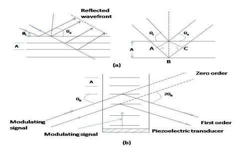
Fig. 4.8. Geometry for Bragg (or reflection-type) acousto-optic diffraction grating modulation : (a) incident rays being scattered from successive layers – for constructive interference the path difference AB + BC must equal an integral number of wavelengths  $m\lambda$  and (b) the amount of light 'reflected' into the first order depends on the amplitude of the modulation signal.
