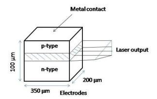
Fig. 3.20 Three-layered laser diode.
