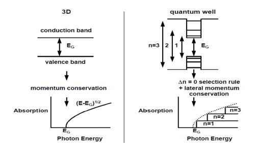
Fig. 2.15: Optical absorption in bulk (i.e., 3D) semiconductors and in quantum wells.
