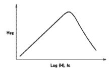
Fig.4.23 Transistor Gain vs Light Intensity
