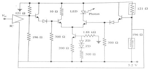
Fig.3.16 An emitter coupled drive circuit which is compatible with ECL
