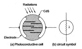
Fig. 4.10 Geometry of the photoconductive cell
