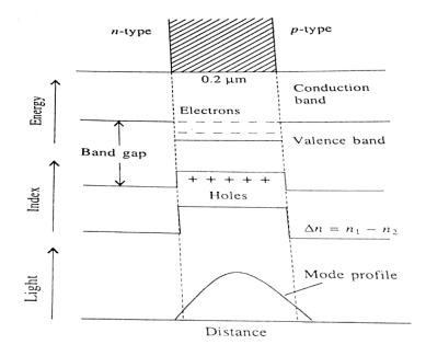
Fig.3.22 Schematic illustration of the simultaneous confinement of the charge carriers and photons offered by the heterostructure scheme
