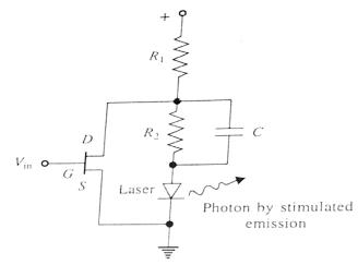
Fig.3.17 A shunt drive circuit for use with an injection laser
