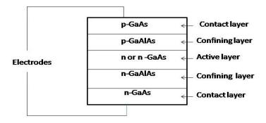
Fig.3.7 Shows 5 layers structure
