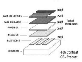
Figure 5.1. Structure of an Electroluminescent Display
