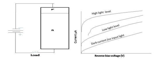
Fig.4.12(a) A typical p-n photodiode (b) characteristics curves
