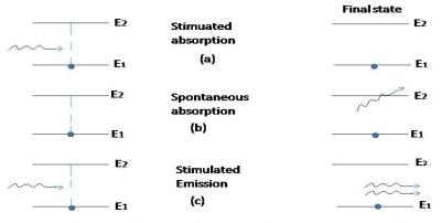
Fig. 1.1. Energy level diagram illustrating (a) stimulated absorption (b) spontaneous emission and (c) stimulated emission. The black dot indicates the state of the atom before and after the transition.
