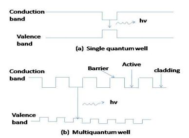
Fig.3.27 Energy band diagrams showing various types of quantum well structure
