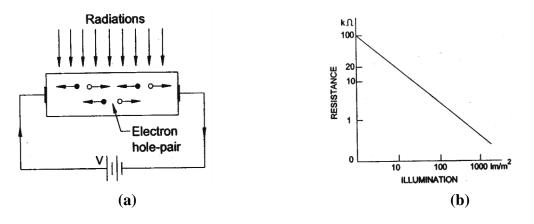
Fig.4.11 (a) Photoconductor in circuit (b) Spectral response of CdS cell
