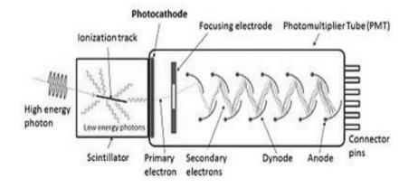
Fig.4.19 Schematic of a photomultiplier tube coupled to a scintillator. This arrangement is for detection of gamma rays.
