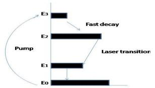
Fig. 1.3 Population of energy levels in a four level system. Population inversion is achieved by pumping to a high energy state  $(E_3)$  followed by fast decay to a lower energy state  $(E_2)$  which happens to be the upper laser level.
