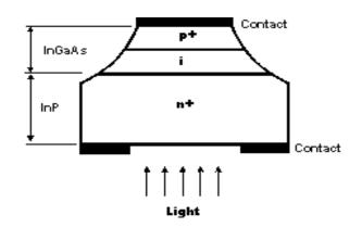
Fig.4.15 PIN photodiode heterojunction structure
