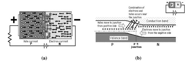
Fig.2.7 Biasing the PN Junction. (a) Forward bias (b) Energy band diagram
