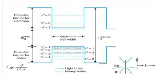
Fig.2.12: One-dimensionally confined quantum well created by a thin small-band gap semiconductor layer sandwiched between two larger band gap semiconductor layers. Eg <sup>Well</sup> is the band gap of the well material and Eg <sup>barrier</sup> that of the barrier material.
