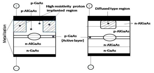
Fig.3.25 Gain guided injection laser
