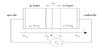
Figure 2.4: Cross-section of a p-n junction
