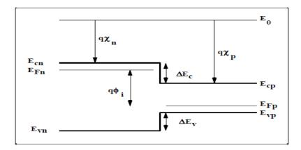
Fig.2.11 Flat band energy band diagram of a p-n junction
