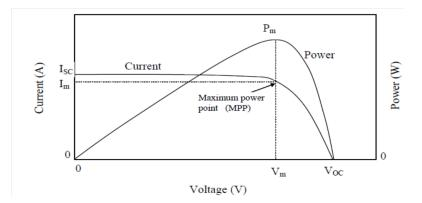
Fig.4.27 I-V Characteristics of solar panel
