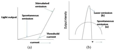
Fig.1.19 (a) Light output – current characteristics of a ideal semiconductor laser (b) Radiant output as a function of frequency for a p-n junction laser.
