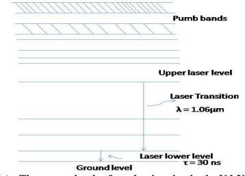
Fig 1.10(a) : The energy levels of neodymium ion in the Nd:YAG laser
