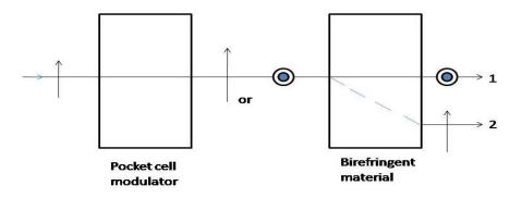
Fig. 4.3 Beam switching using a Pockels cell modulator. As the applied voltage is changed from zero to  $V_{\pi}$  the beam is switched from position 1 to position 2.
