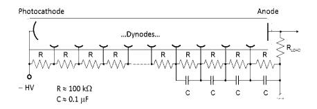
Fig.4.20 Typical photomultiplier voltage divider circuit using negative high voltage.
