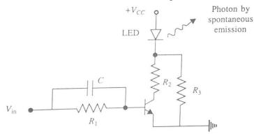
Fig. 3.12 A simple drive circuit for binary digital transmission consisting of a common emitter saturating switch.
