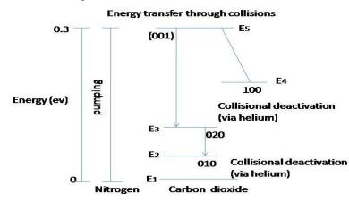
Fig.1.14 Simplified energy level diagram for the CO2 laser
