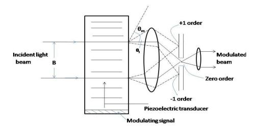
Fig 4.7 Geometry for Raman-Nath (or transmission-type) acousto-optic diffraction grating modulation. The amount of light diffracted into the orders  $m \ge 1$  from the incident beam, and hence the modulation of the transmitted beam, depends on the amplitude of the modulating signal.
