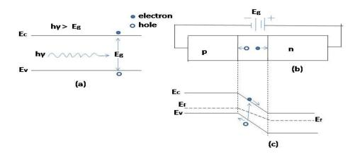
Fig.4.13(a) Operating principle of p-n photodiode (a) photogeneration of an electron hole pair in an intrinsic semiconductor (b) structure of a reverse biased photodiode (c) energy band diagram of the reverse biased p-n junction illustrating photogneration and subsequent of an electron-hole pair
