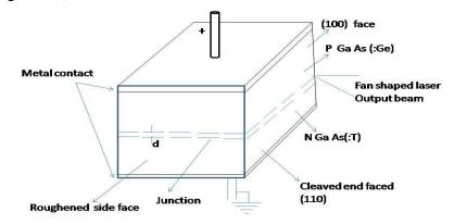
Fig. 1.18 Schematic construction of a *GaAs* homojunction semiconductor diode laser having side lengths 200- -400 μm. The emission is confined to the junction region.
