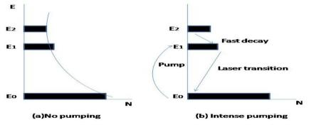
Fig.1.2 Population of energy levels by pumping in a three level system
