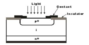
Fig.4.14 PIN photodiode structure
