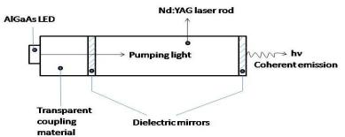
Fig.1.10(b) Schematic diagram of an end pumped Nd:YAG laser
